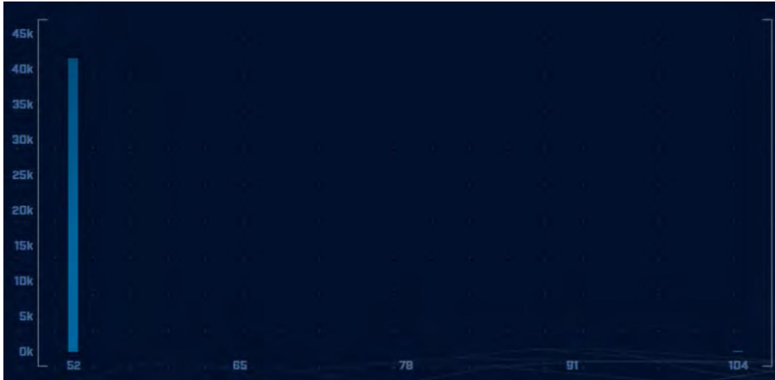
**This example shows the number of connections transferring amounts of data. In this case approximately 42,000 connections transferred 52 bytes of data over a 24-hour period.**
